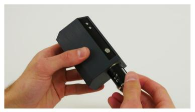
2) Use the pipette to inject 1-2 drops of fog liquid inside the silver heating coil
