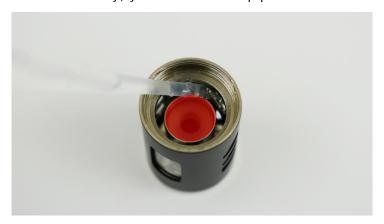
4) Screw the fluid tank back on and allow the liquid to soak into the heating element by not using it for 10-15 mins. The priming process is now complete
