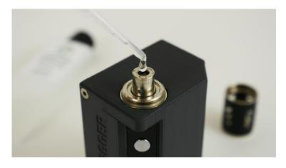
3) Fill up the fluid tank using the pipette. Be careful to not get any liquid into the central cavity as this will result in small leaks later on. Only fill the liquid up to the top rim of the central cavity, you can use the pipette to measure out 2ml of fluid.
